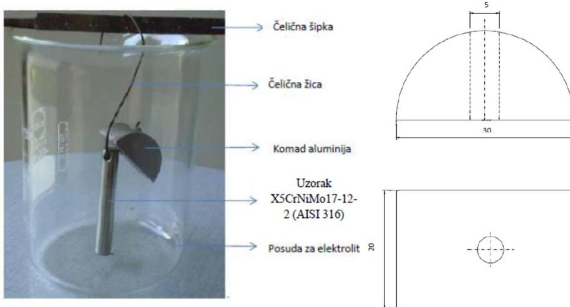
Slika 4.52. Uzorak čelika X5CrNiMo17-12-2 u dodiru
