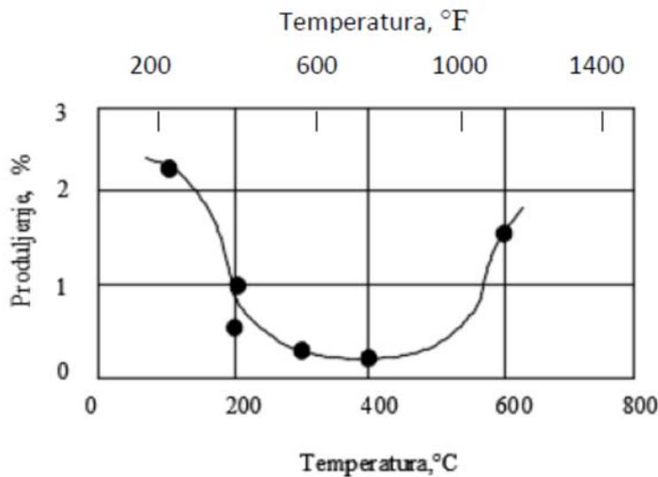
Slika 2.18. Utjecaj toplinske obrade na duktilnost Ni-P prevlake (The Engineering Properties of Electroless Nickel Coatings, 1980).
