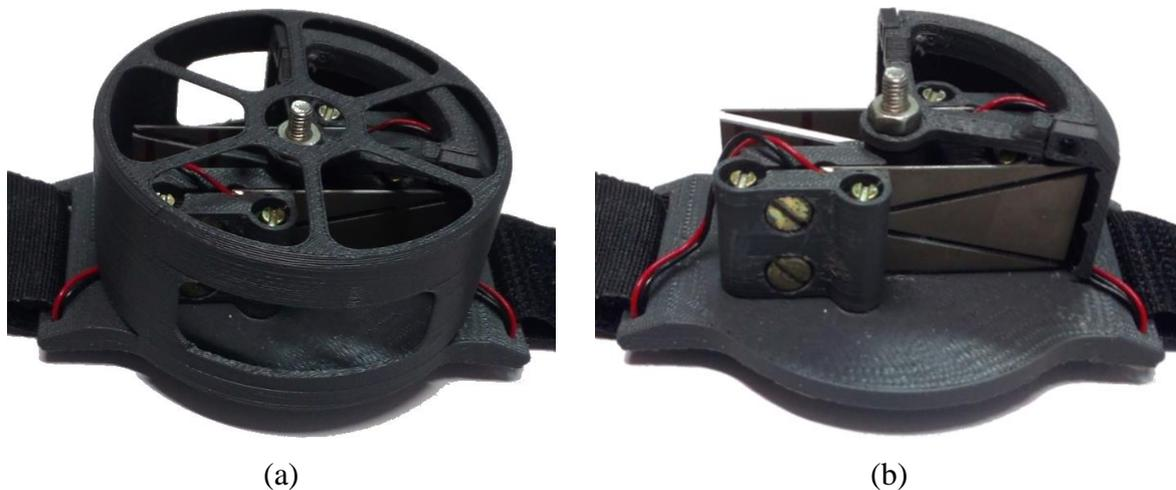
Figure 7.15. 3D printed demonstration model of the devised wearable device prototype with (a) and without the protective cover (b).
