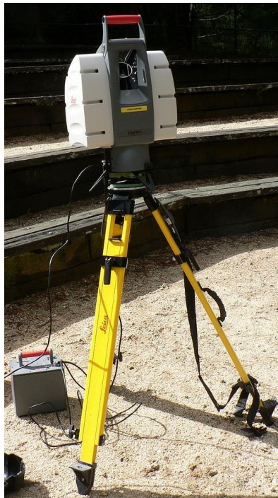
Slika 2.2 Time of Flight skener [4]
