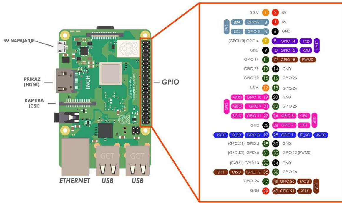
Slika 2.1.3 Raspberry Pi v3 PIN layout [22]
