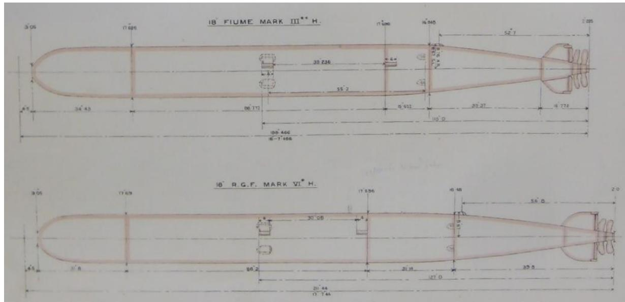
Slika 4.17. Nacrt – 18in Fiume Mark III\*\* H torpedo
