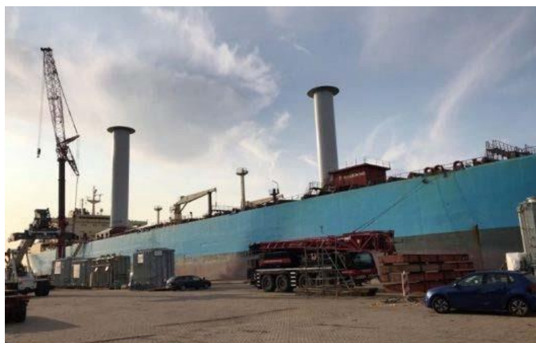
Figure 2. Flettner rotors on board Maersk Pelican, [21]
