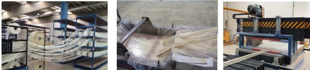
Figure 23 Extruded profiles production facilities
