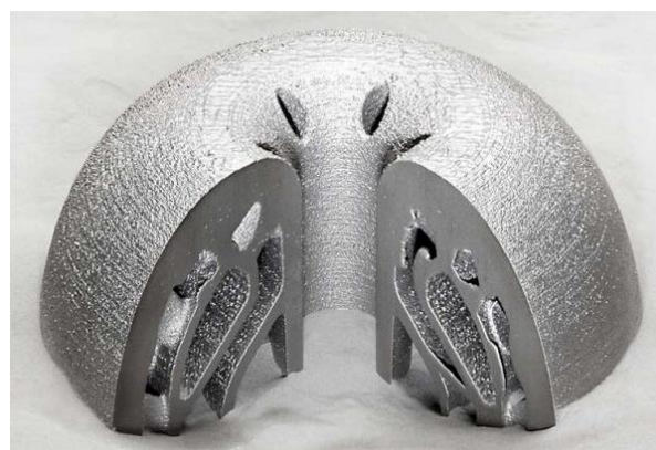
Figure 5. A probehead for taking gas samples in hot gas atmosphere, produced at the Thyssenkrupp TechCenter Additive Manufacturing [15]
