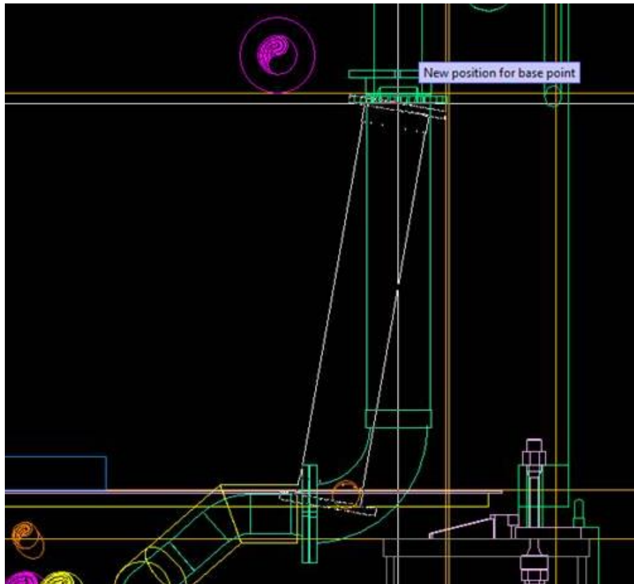
Figure 15 Engine and hose connection – compromise solution
