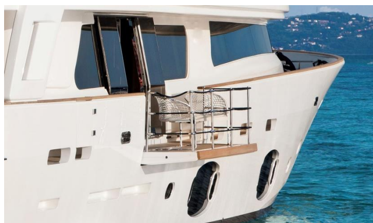
Figure 8 Transformable systems for balcony bulwark
