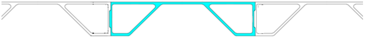
Figure 31 Pultruded profile geometry
