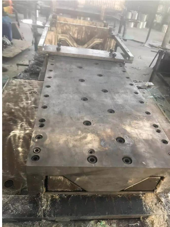
Figure 44 Pultrusion process – RAMSSES forming dye
