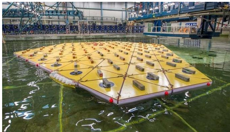
Figure 12 Testing an innovative concept for a floating mega-island, MARIN, [8]
