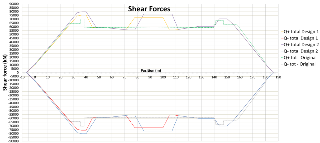
Figure 81 Comparison of shear forces Design 1,2 + Original Vessel
