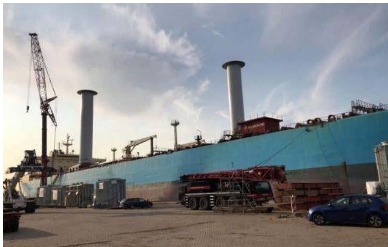
Figure 2. Flettner rotors on board Maersk Pelican, [21]
