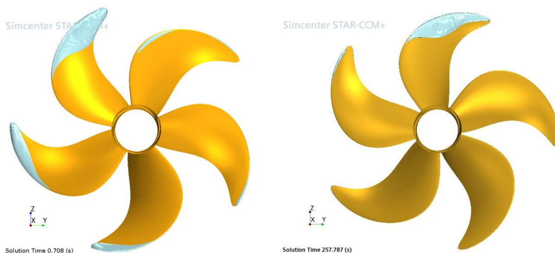
Figure 15 Iso-surfaces of 5% vapor volume fraction on propeller blades: model scale (left) and full scale (right).
