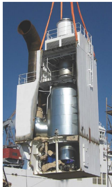
Figure 118 Preassembled section with Alfa Laval's scrubber unit
