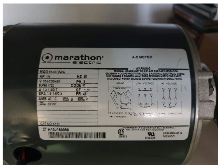
Slika 10.1. Marathon electric 5K33GN2A asinkroni elektromotor
