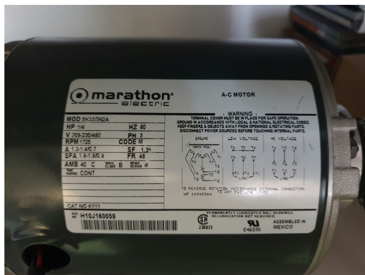
Slika 10.1. Marathon electric 5K33GN2A asinkroni elektromotor
