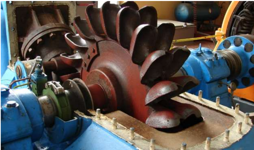
Slika 5.5. Peltonova turbina (preuzeto sa: https://housing.com/news/pelton-wheel-turbine-meaning-design-operations-components-applications-advantages-and-disadvantages/ )
