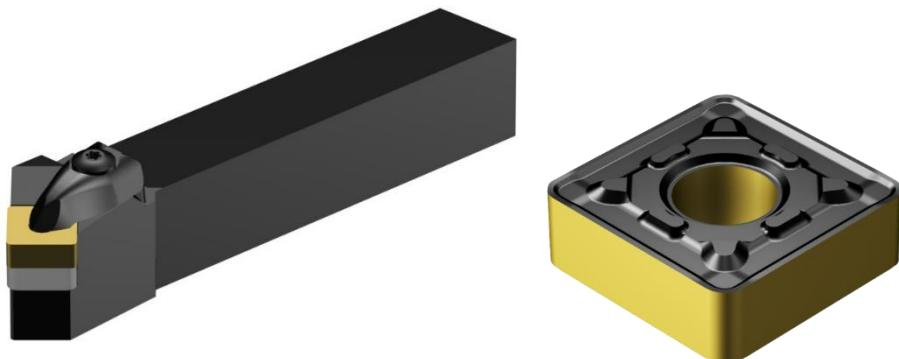
Slika 5.2 Tokarski nož DSSNR 2525M 15 s pločicom SNMG 15 06 08-PR 4415 [7]
