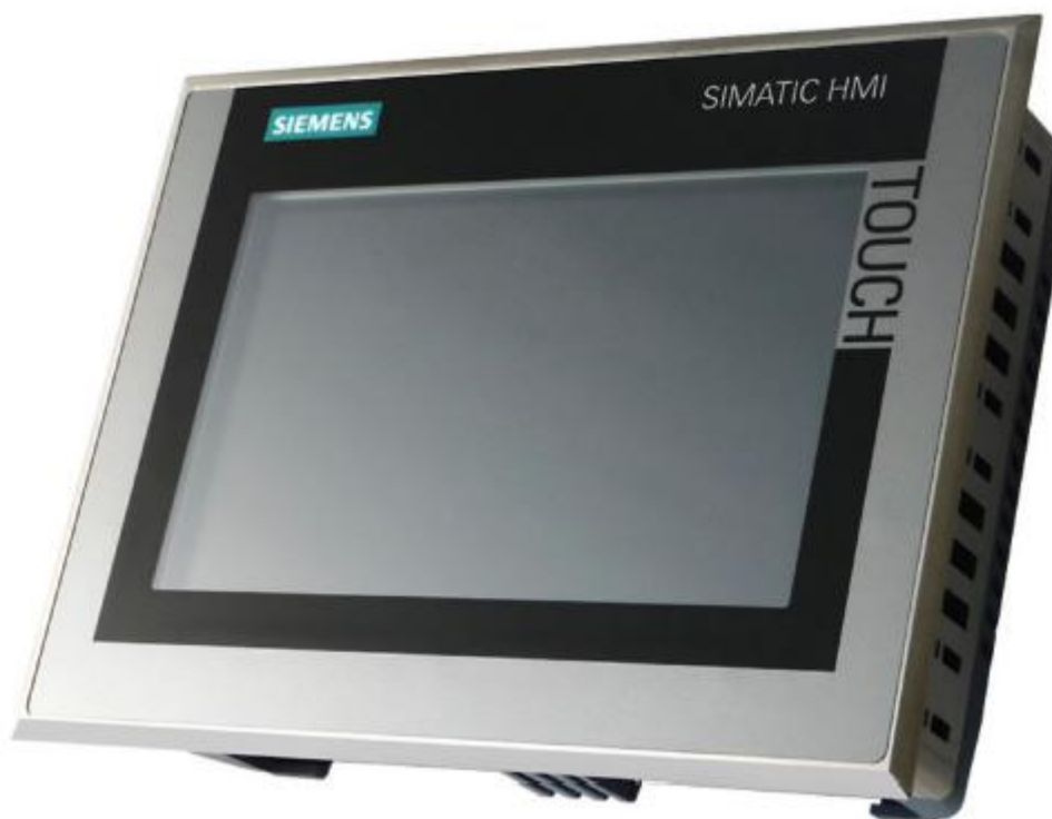
Slika 4.1. TP900 Comfort HMI panel [8]
