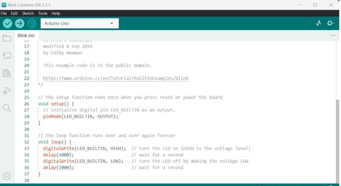
The screenshot shows the Arduino IDE interface with the title bar "Blink | Arduino IDE 2.1.1". The menu bar includes File, Edit, Sketch, Tools, and Help. The board selector dropdown shows "Arduino Uno". The code editor displays the "Blink.ino" sketch. The code is as follows:
