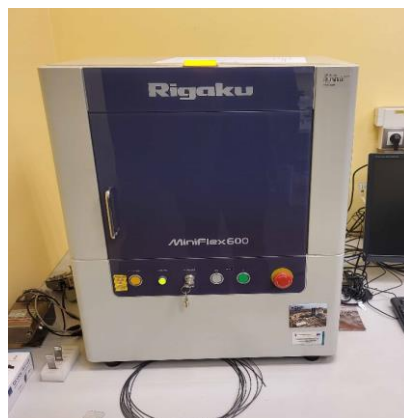
Figure 26. Rigaku MiniFlex 600 diffractometer
