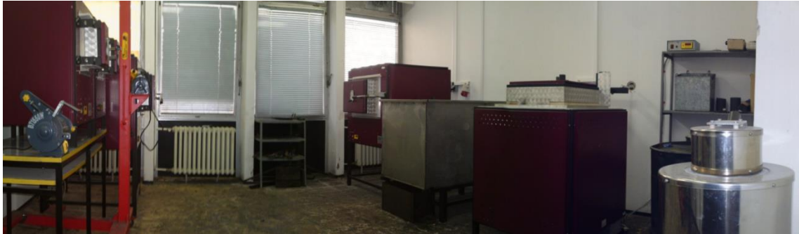
Figure 21. OVER furnaces for heat treatment of SMA alloys
