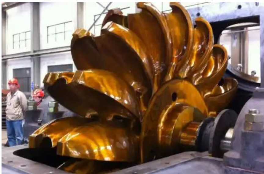
Slika 3.4 Lopatice Peltonove turbine [20]
