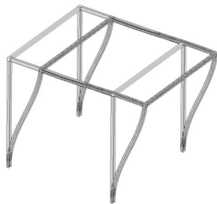
Figure 7. Sway buckling mode – shell model NASTRAN.
