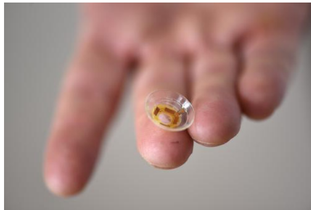
Fig.7 - The first stand-alone contact lens with a flexible micro battery.
