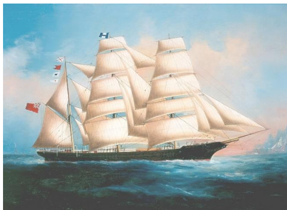
Figure 1 A barque with square sails on foremast and mainmast, the rest are fore-and-aft sails Slika 1 Bark s križnim jedrima na pramčanom i prednjem jarbolu i letnim jedrima na ostalim jarbolima (Source/Izvor: Anonymous - Vallejo Gallery, Public Domain, https://commons.wikimedia.org/w/index.php?curid=79161068 )
