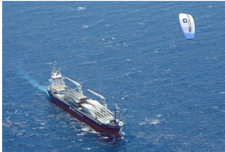
Figure 1. Towing kite system, [20]
