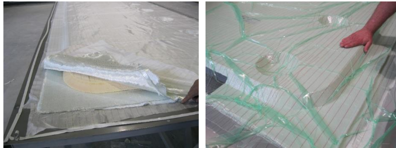
Figure 17 Composite sandwich panel
