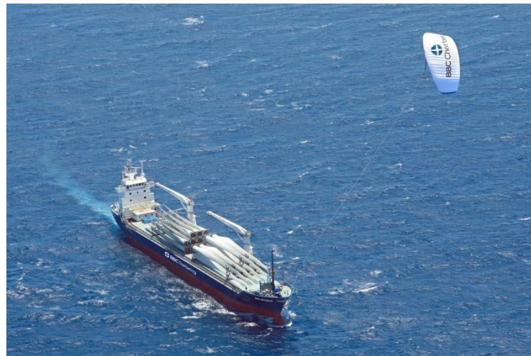
Figure 1. Towing kite system, [20]
