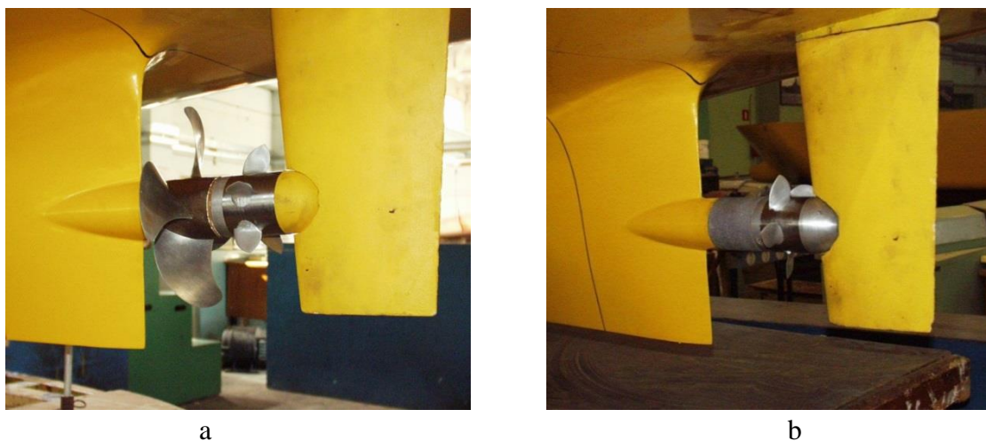
Figure 3 The TSMP model with contra propeller installed behind the hull of the tested model: a- energy-saving mode, full speed simulation, see fig.1a; b – slow speed simulation, see fig.1c
