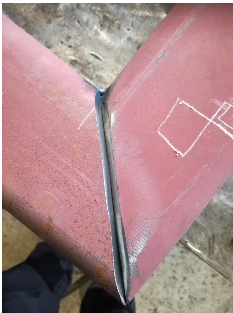
Slika 3 – Square profile joint preparation in production
