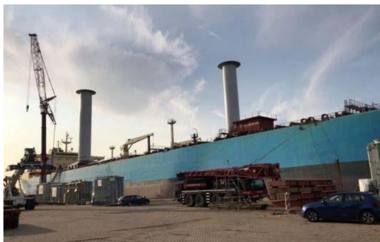
Figure 2. Flettner rotors on board Maersk Pelican, [21]
