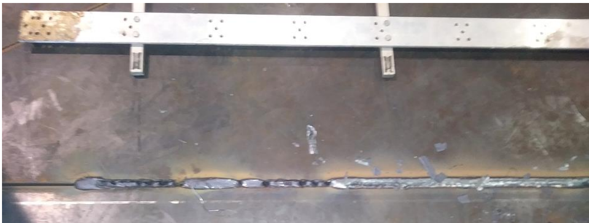
Figure 12 insufficient filling due to greater distances between “leaflets”
