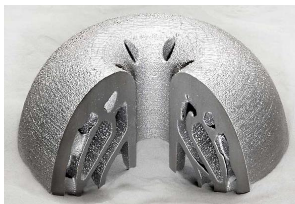
Figure 5. A probehead for taking gas samples in hot gas atmosphere, produced at the Thyssenkrupp TechCenter Additive Manufacturing [15]
