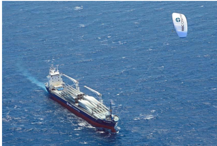
Figure 1. Towing kite system, [20]
