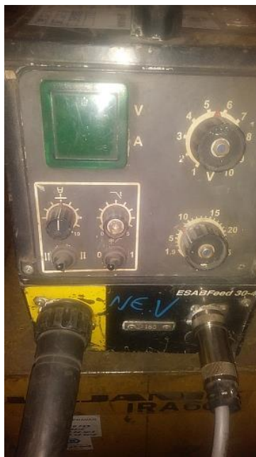
Figure 3 wire system control
