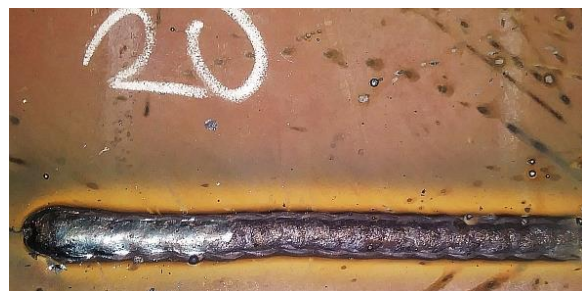
Figure 7 insufficient weaving overlap, weld 20
