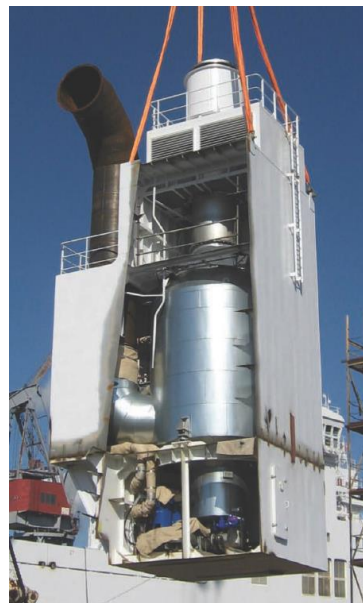
Figure 118 Preassembled section with Alfa Laval's scrubber unit
