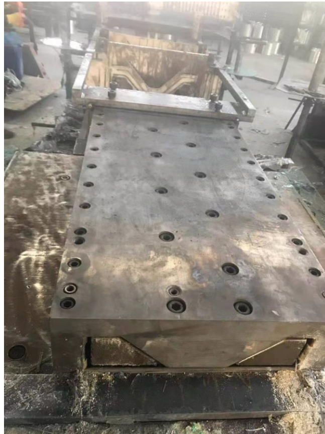
Figure 44 Pultrusion process – RAMSSES forming dye
