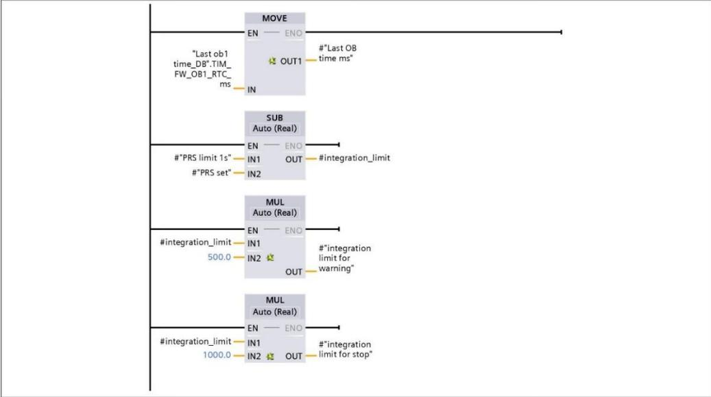
**Network 2:** If pressure is above set, calculate difference and integrate, integration resets after each movement end
