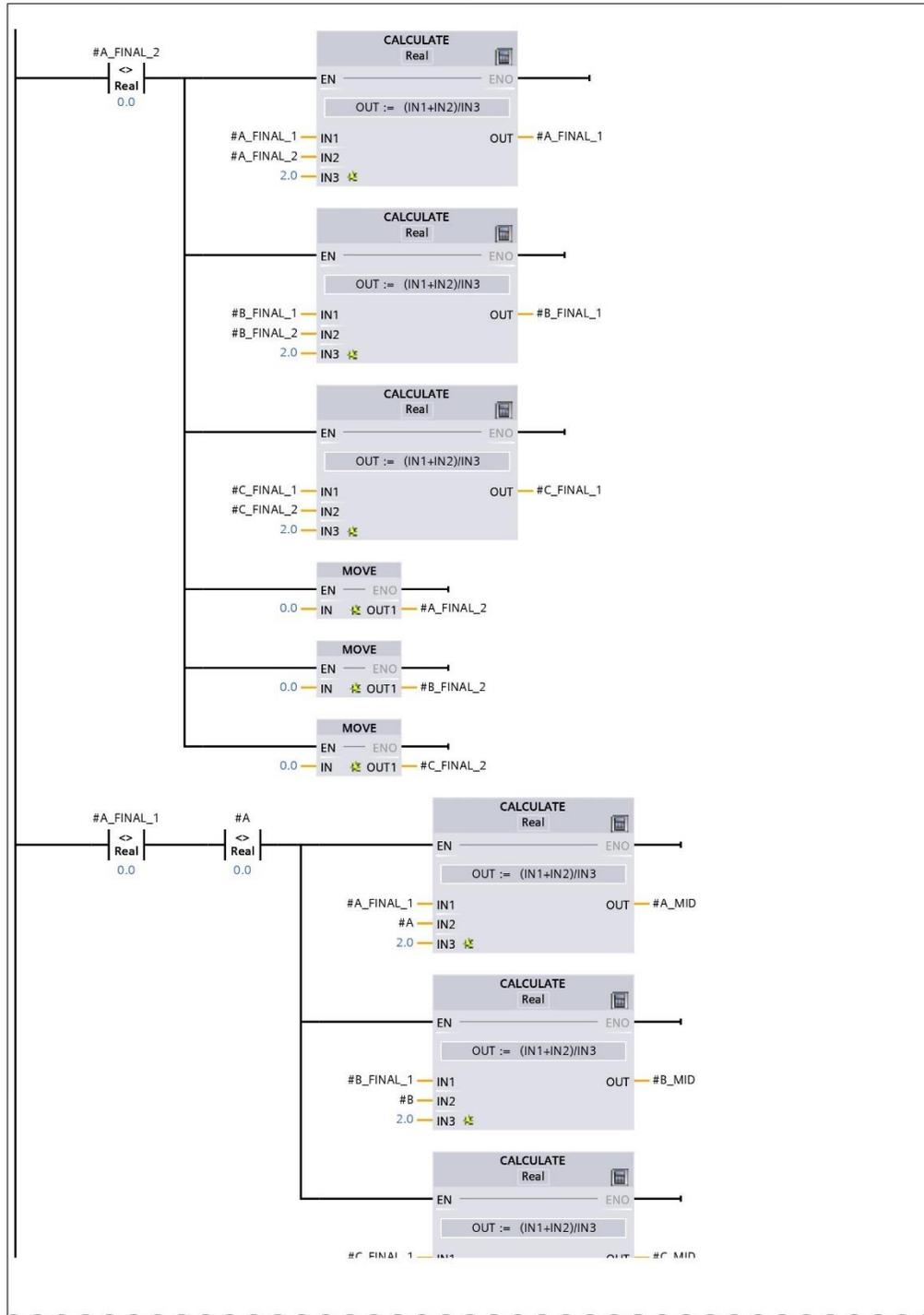
Network 12: CALCULATES AVERAGE OF 2 LAST FINAL COEFICIENTS (2.1 / 2.1)
