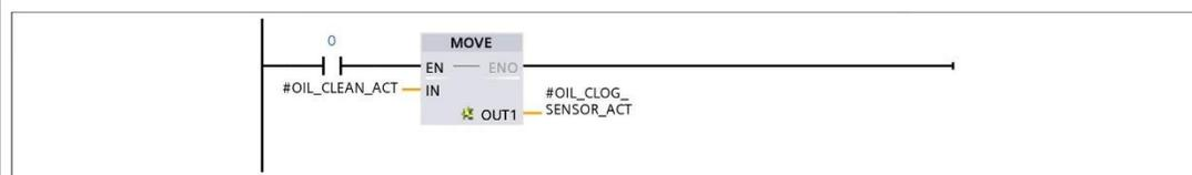
**Network 2: TAKING NEXT SAMPLE (EVERY 24H OF MACHINE RUNNING TIME, WHILE OIL TEMP IN SPECIFIC RANGE)**
