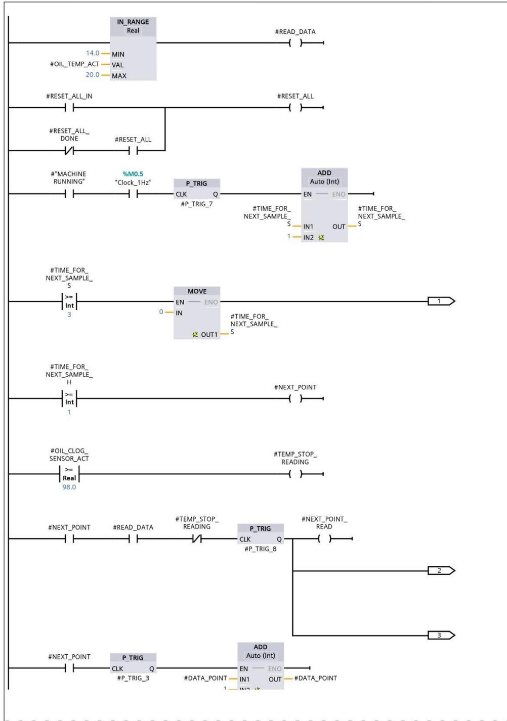
Network 2: TAKING NEXT SAMPLE (EVERY 24H OF MACHINE RUNNING TIME, WHILE OIL TEMP IN SPECIFIC RANGE) (;
