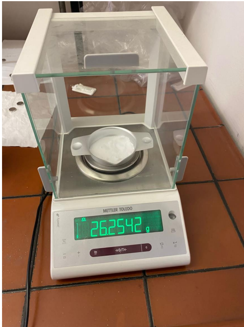
Slika 4.2.: Vaga Mettler Toledo NewClassic MF JP703C
