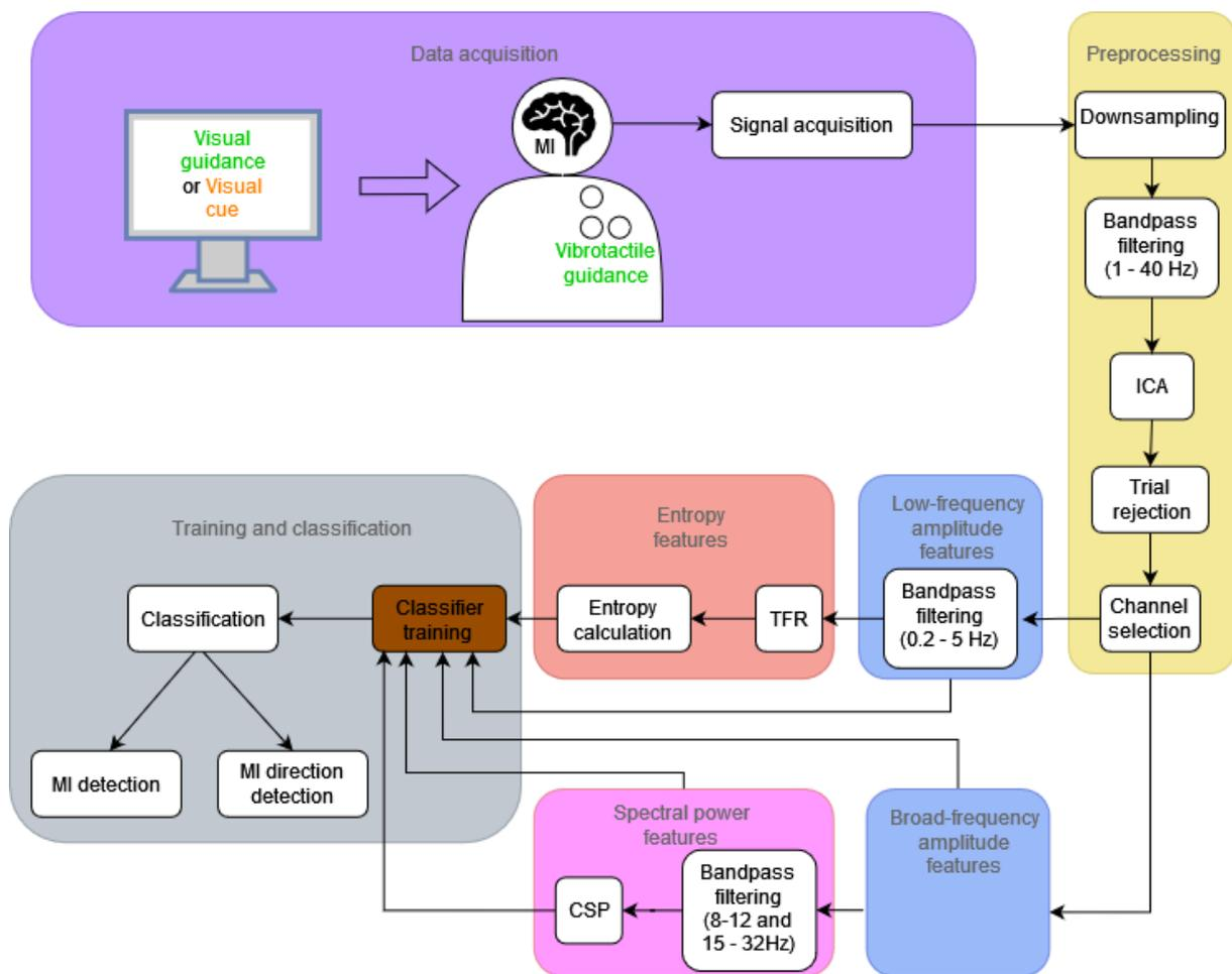
**Figure 4.2:** Flowchart of the processing pipeline [33].
