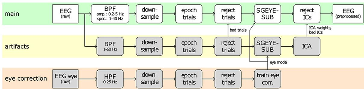
**Figure 4.1:** Common preprocessing techniques that were applied to EEG signals in this research. The uppermost branch, colored green, depicts the primary preprocessing techniques that were implemented on the trials. The lower branches illustrate the methods utilized to remove eye artifacts (colored in orange at the bottom) and general artifacts (colored in yellow in the middle) [1].
