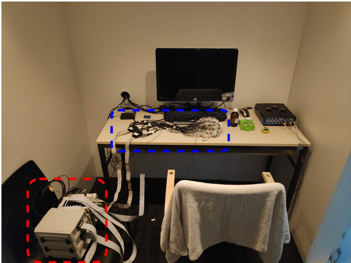
**Figure 1.3:** An example of a BCI system utilizing EEG. The amplifiers are marked with a red rectangle, and the active electrodes and cap are marked with a blue rectangle. During the experiment, the subject sits on the chair in front of the screen, and the screen displays cues and instructions about the experiment.
