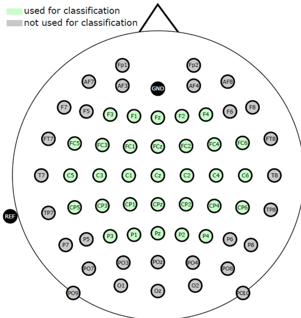
**Figure 3.3:** International 10/20 EEG system cap montage [1].
