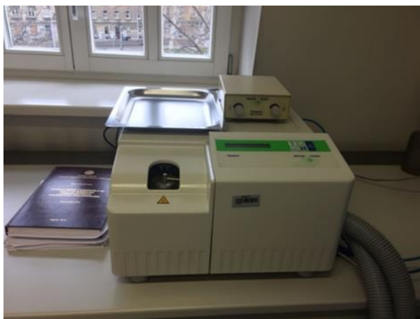
Figure 29. Mettler-Toledo 822e MDSC
