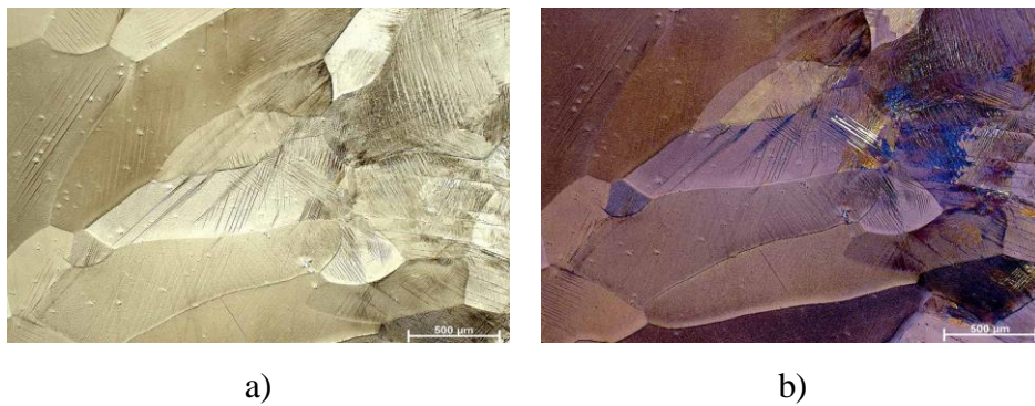
Figure 46. OM micrographs of quenched Cu-9Al-10Mn-2Ag SMA alloy: a) BF, mag. 50x, b) POL, mag 50x
