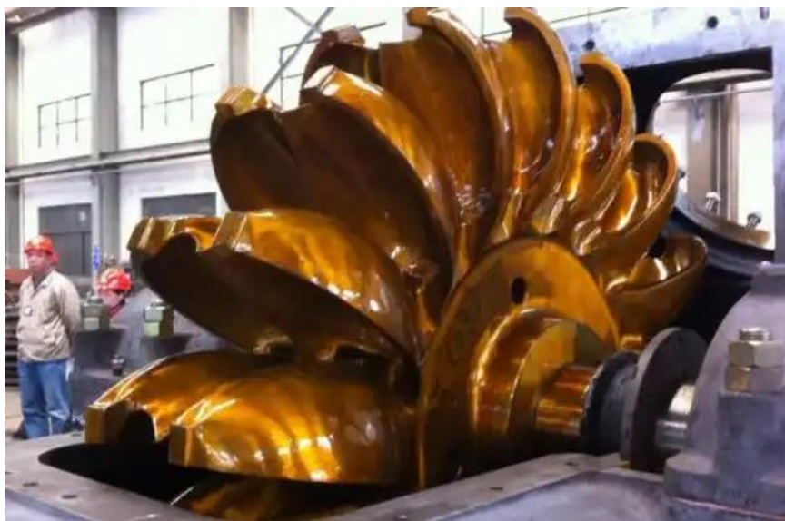
Slika 3.4 Lopatice Peltonove turbine [20]
