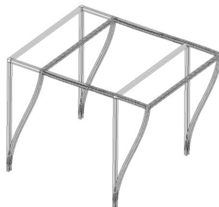
Figure 7. Sway buckling mode – shell model NASTRAN.
