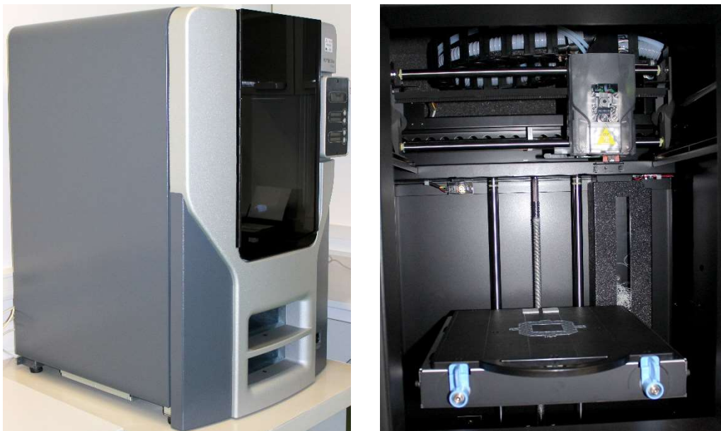
Figure 2.3. Stratasys Fortus 250mc 3D printer at the LPEMNST – CMNST of the University of Rijeka
