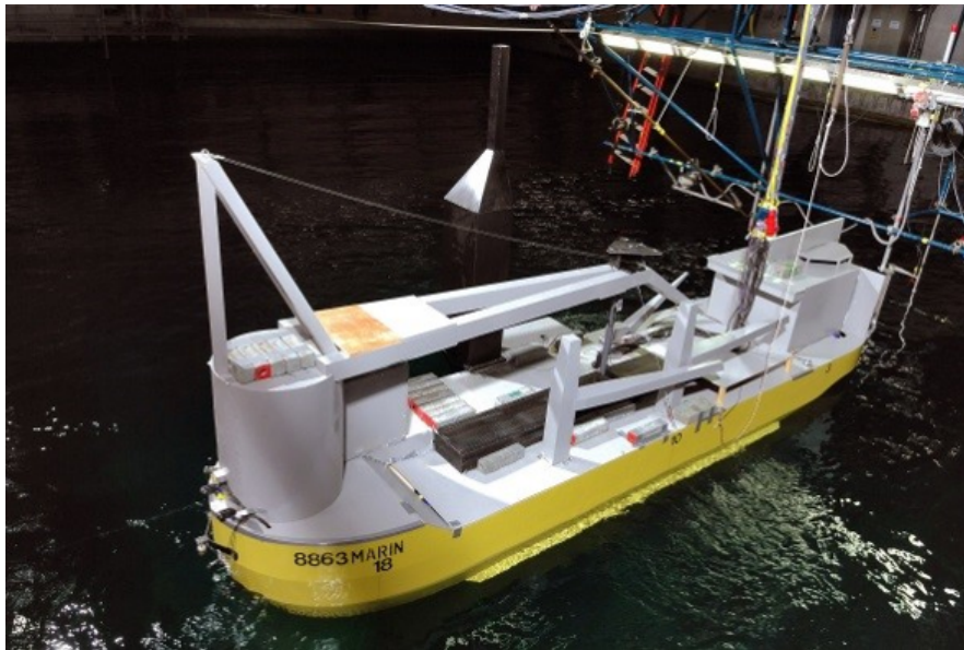
Figure 4.25: PLCV model during current loads test at MARIN
