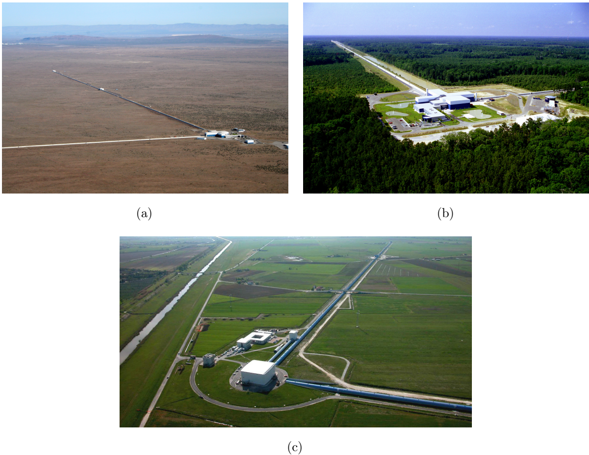
Figure 4.2 GW detector sites: (a) LIGO Hanford [160]; (b) LIGO Livingston [161]; (c) Virgo [162]. Courtesy Caltech/MIT/LIGO Laboratory and Virgo Collaboration.
