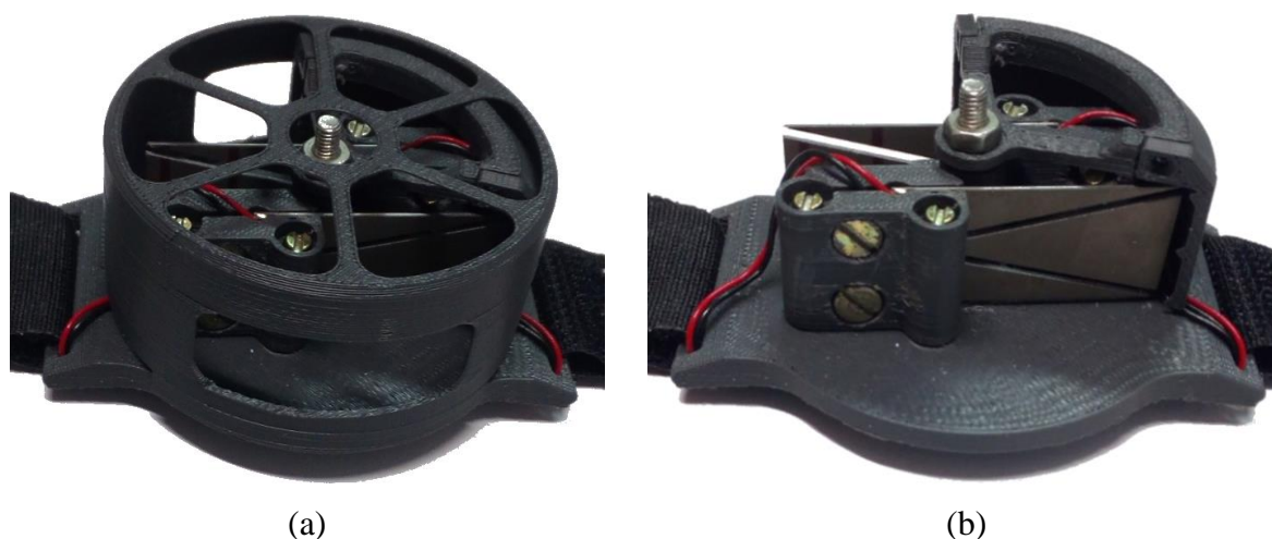
Figure 7.15. 3D printed demonstration model of the devised wearable device prototype with (a) and without the protective cover (b).
