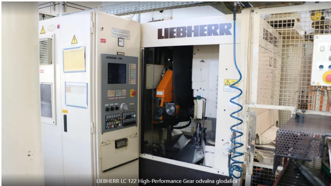
Slika 5.38 LIEBHERR LC 122 High-Performance Gear odvalna dubilica
