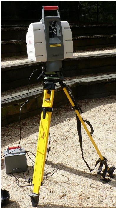
Slika 2.2 Time of Flight skener [4]
