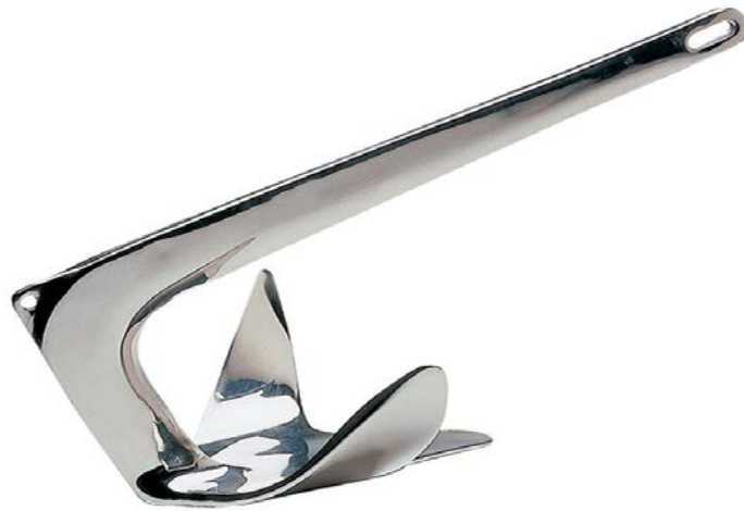
Slika 3.1.1.: Lewmar 110 lb. Stainless-steel Claw Anchor
