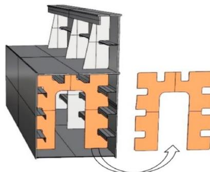
Fig. 1. Upper wing torsional box. Transverse web detail.
