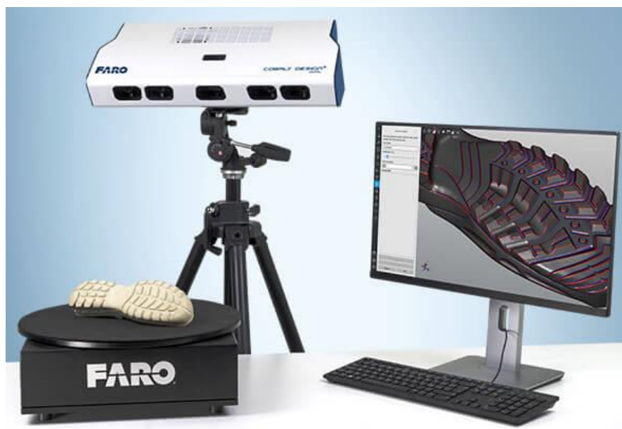
Slika 3.1 Skener FARO Cobalt Design Dual [6]
