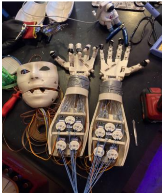
Figure 3. Fully assembled hands and finger
