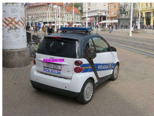
Figure 2. Output image of the YOLO algorithm after successful detection
