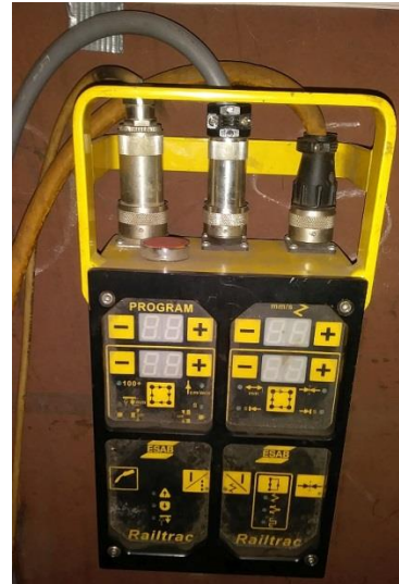
Figure 2 control box detail
