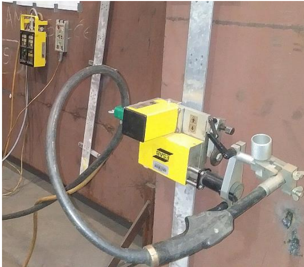
Figure 1 welding carriage system
