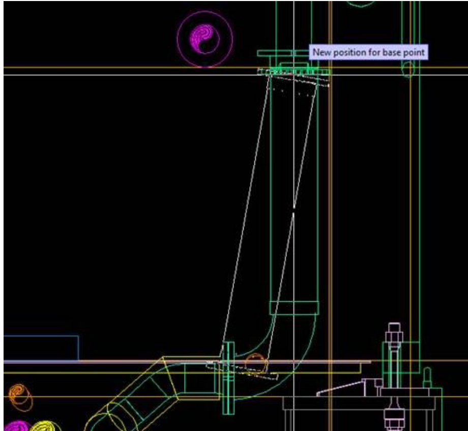
Figure 15 Engine and hose connection – compromise solution
