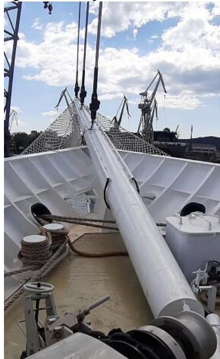
Figure 9 Bowsprit connection to deck and stem Slika 9 Spoj pramčanog kosnika na palubu i statvu
