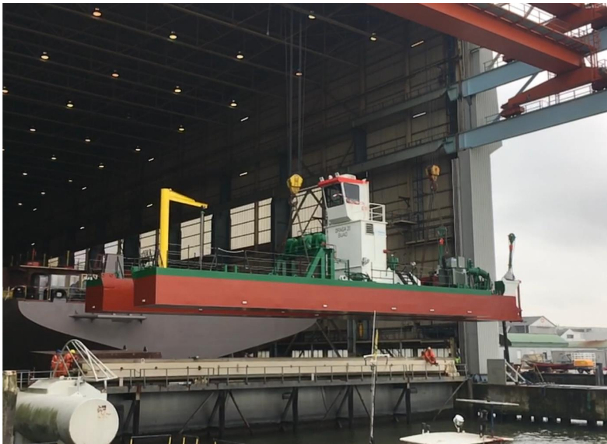
Figure 6 Lowering the dredger for the first time into water in the Shipyard
