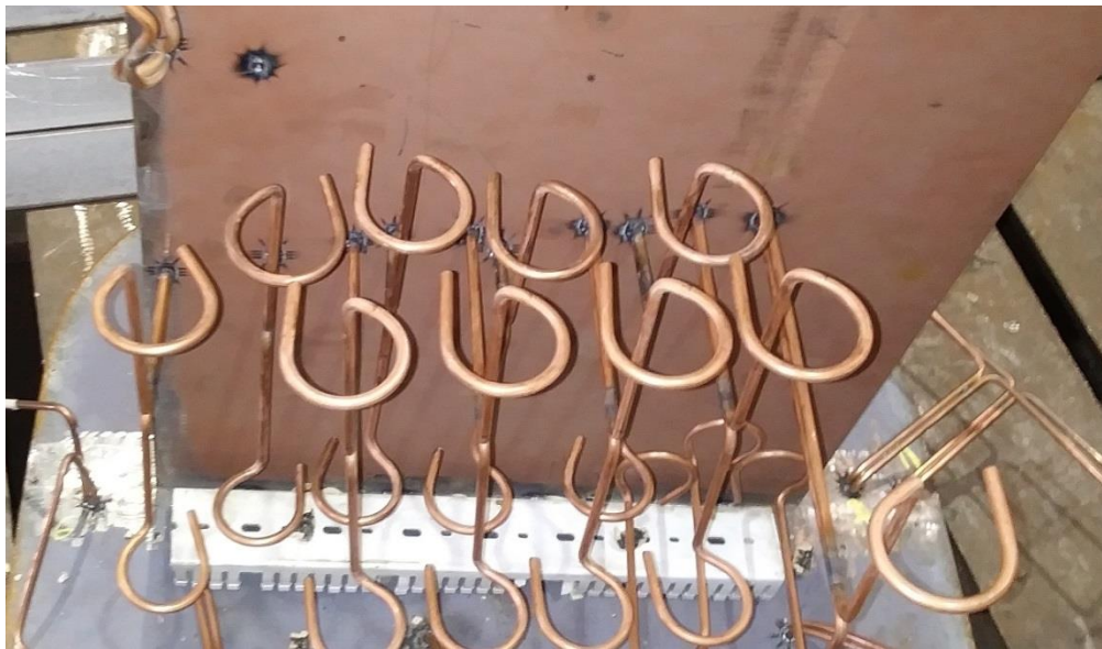
Figure 6 Tenfold cable holder positioning on 4 levels. Upper level consist of 4 HDO 60 cable holders, below them are 4 HDO 150, left of them is HDO 100 and in lower right corner HDO 250
