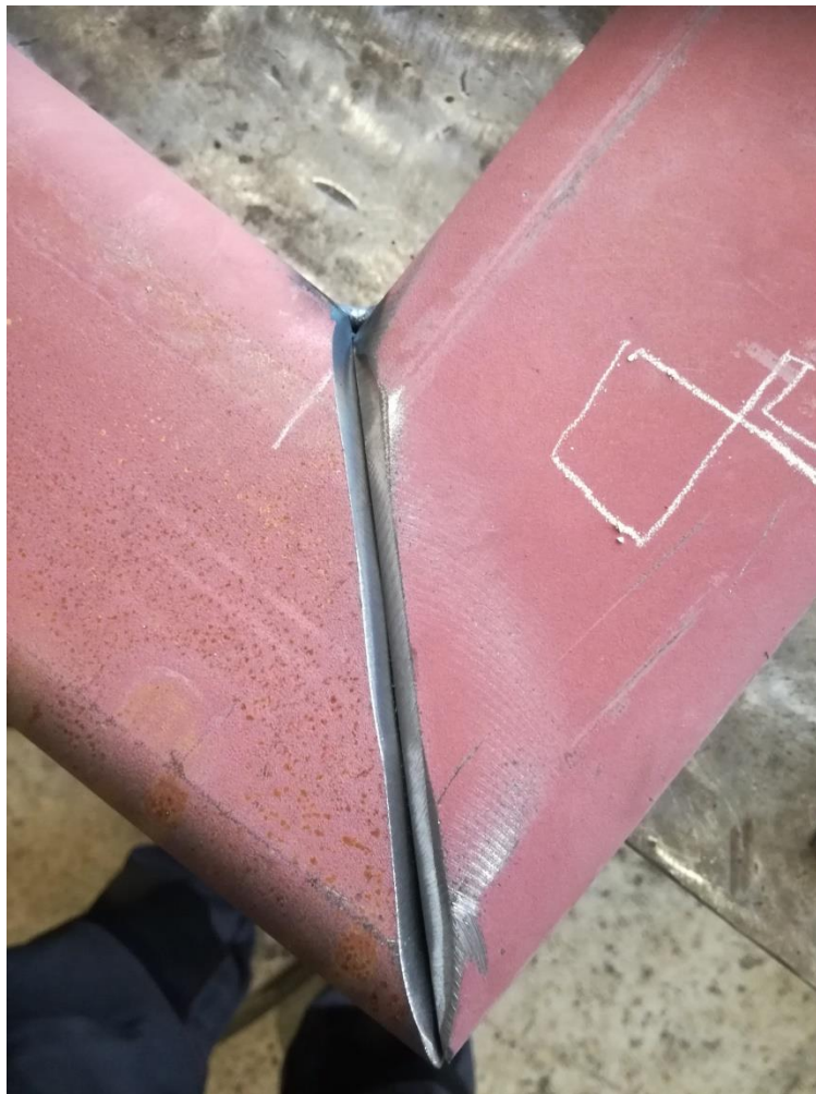
Slika 3 – Square profile joint preparation in production
