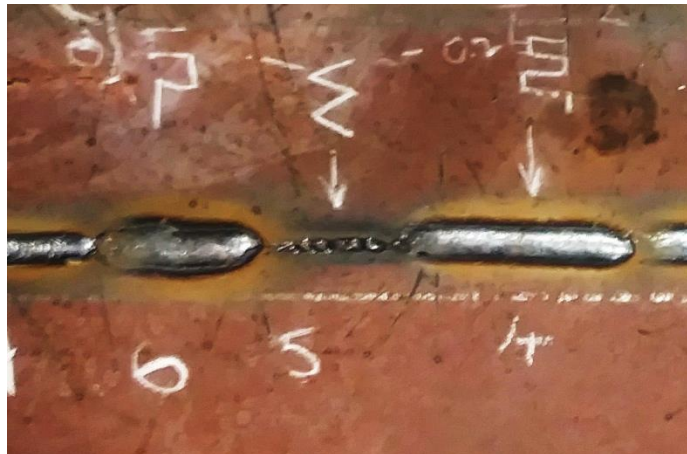
Figure 9 difference in weaving types, zig-zag vs. interrupted weaving Slika 9 razlika u načinu njihanja; cik-cak u odnosu na isprekidano
