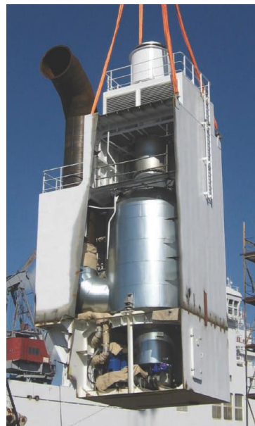
Figure 118 Preassembled section with Alfa Laval's scrubber unit
