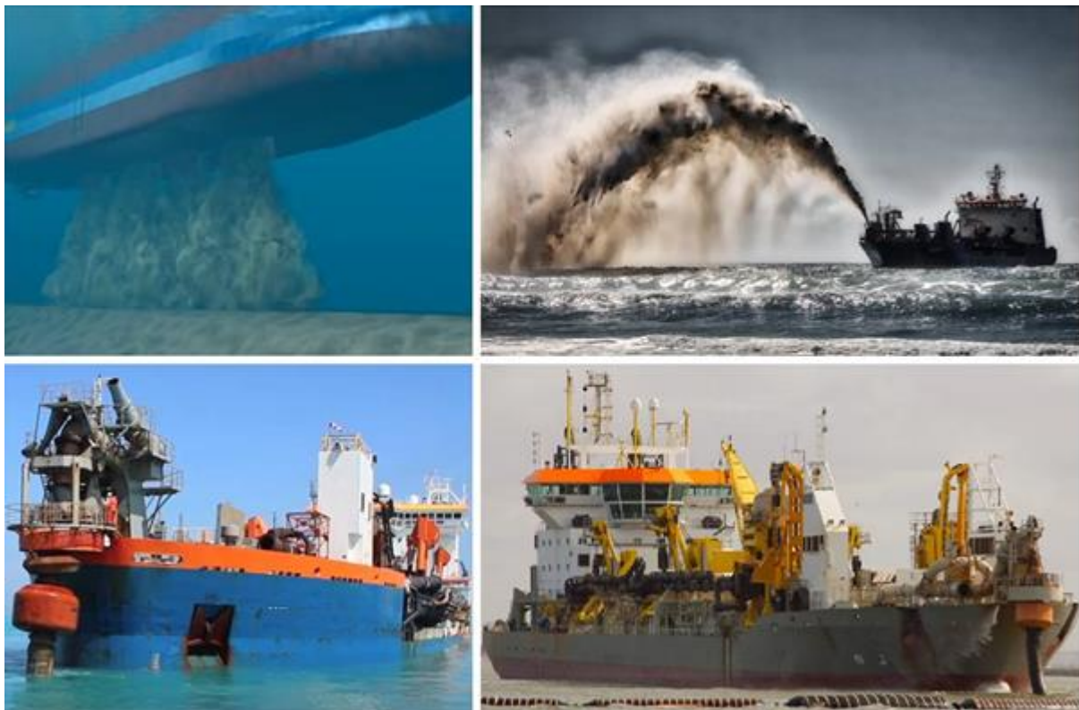
Figure 52 Images of typical means of Hopper Discharging; From left to right – Bottom Doors; Rainbowing; Bow coupling connected to floating pipeline
