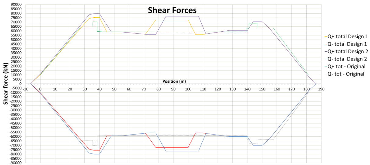
Figure 81 Comparison of shear forces Design 1,2 + Original Vessel
