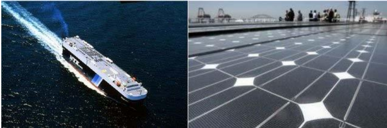
Figure 3. NYK car carrier “Auriga Leader” (left), solar panels on the top deck (right), [24]
