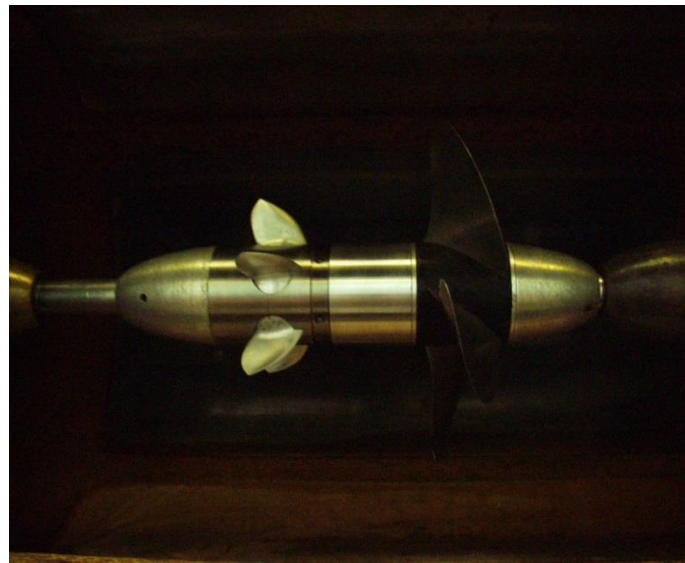
Figure 2 Model of TSMP with contra propeller in the working section of KTSP, energy-saving mode, see fig. 1a
