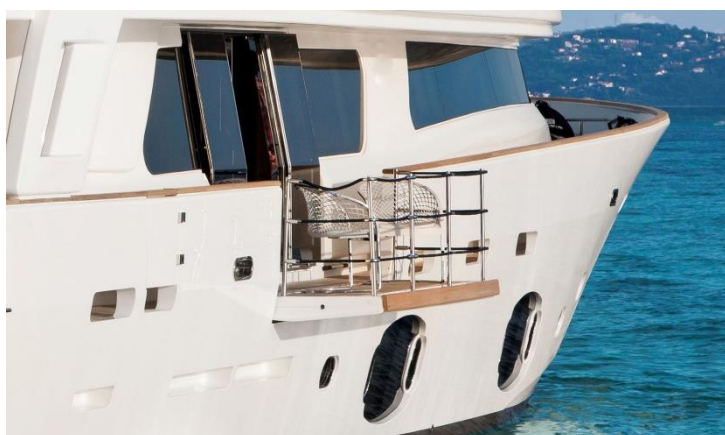
Figure 8 Transformable systems for balcony bulwark
