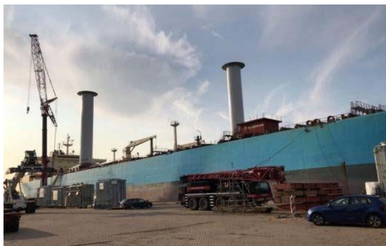
Figure 2. Flettner rotors on board Maersk Pelican, [21]
