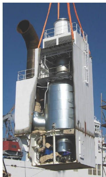
Figure 118 Preassembled section with Alfa Laval's scrubber unit
