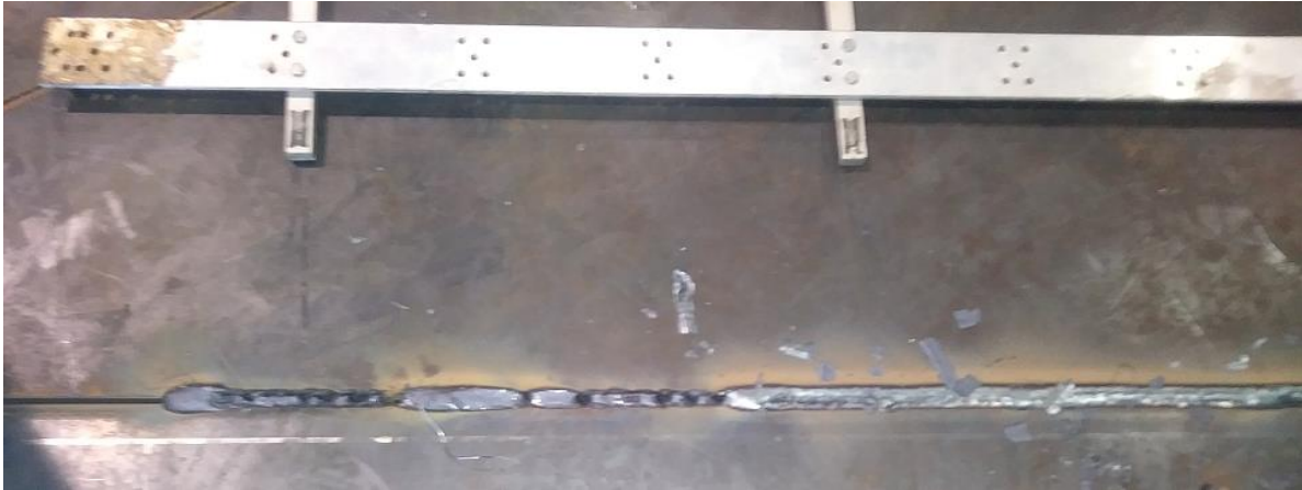
Figure 12 insufficient filling due to greater distances between “leaflets”
