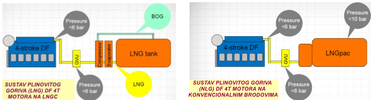
Figure 8 Fuel gas (LNG) systems of DF 4T engines on the LNGC and on gas fuelled ships [8] Slika 8 Sustavi plinovitog goriva (LNG-a) DF 4T motora na LNGC i konvencionalnim brodovima [8]
