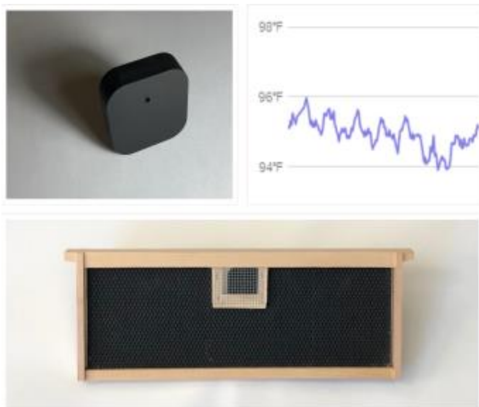
Slika 4.2 HM-1 Smart hive temp/humidity sensor [21]
