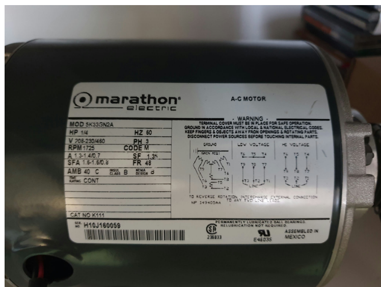
Slika 10.1. Marathon electric 5K33GN2A asinkroni elektromotor
