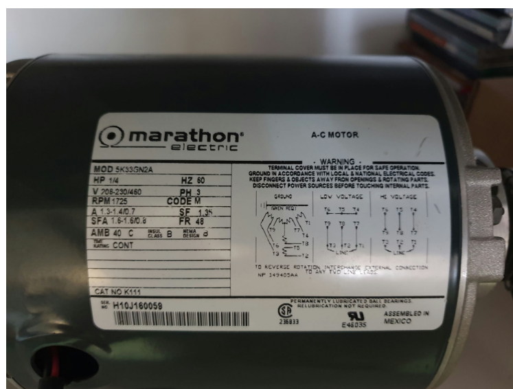
Slika 10.1. Marathon electric 5K33GN2A asinkroni elektromotor
