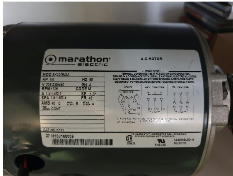
*Slika 10.1. Marathon electric 5K33GN2A asinkroni elektromotor*
