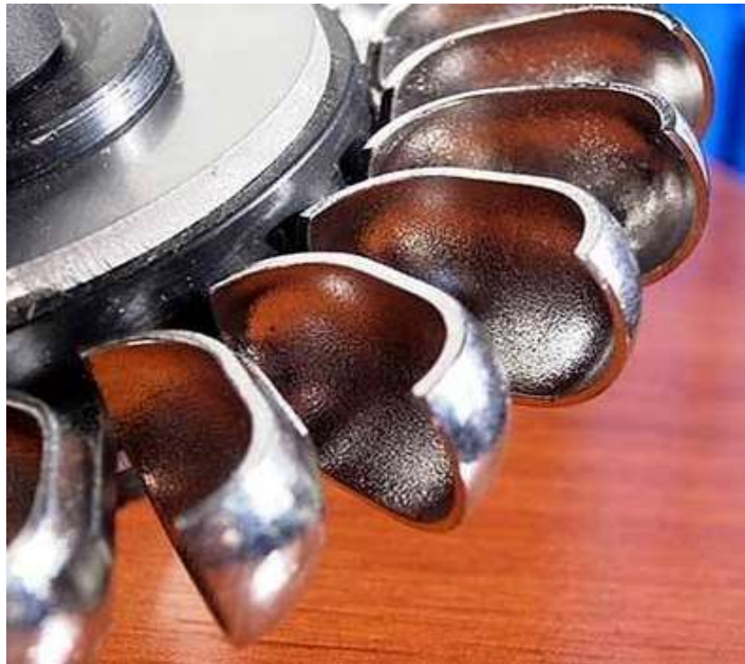
Slika 5.6. Lopatice Turgo turbine (preuzeto sa: https://www.renewablesfirst.co.uk/wp-content/uploads/Stainless-steel-buckets-on-a-DIY-Turgo-turbine.jpg )
