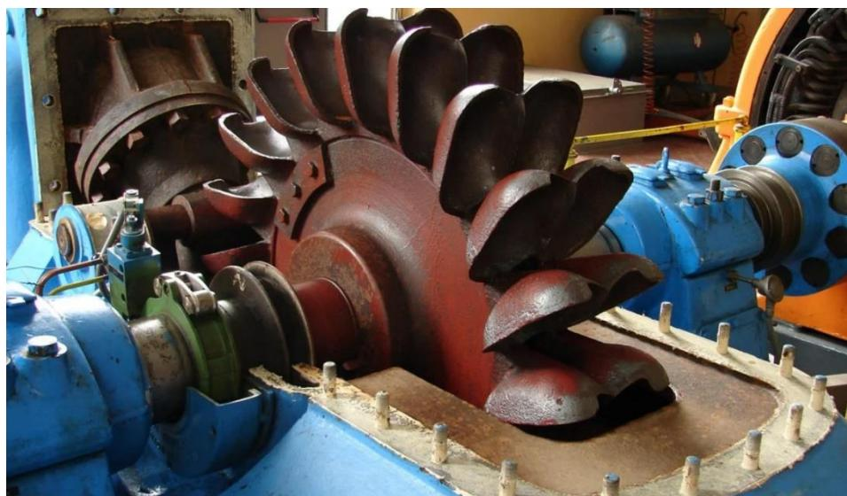
Slika 3.2. Pelton turbina [8]
