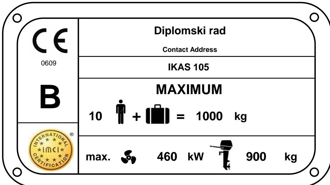
Builder's plate information for craft powered by inboard or sterndrive engines
