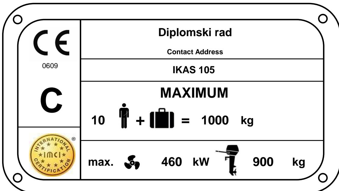
Builder's plate information for craft powered by inboard or sterndrive engines
