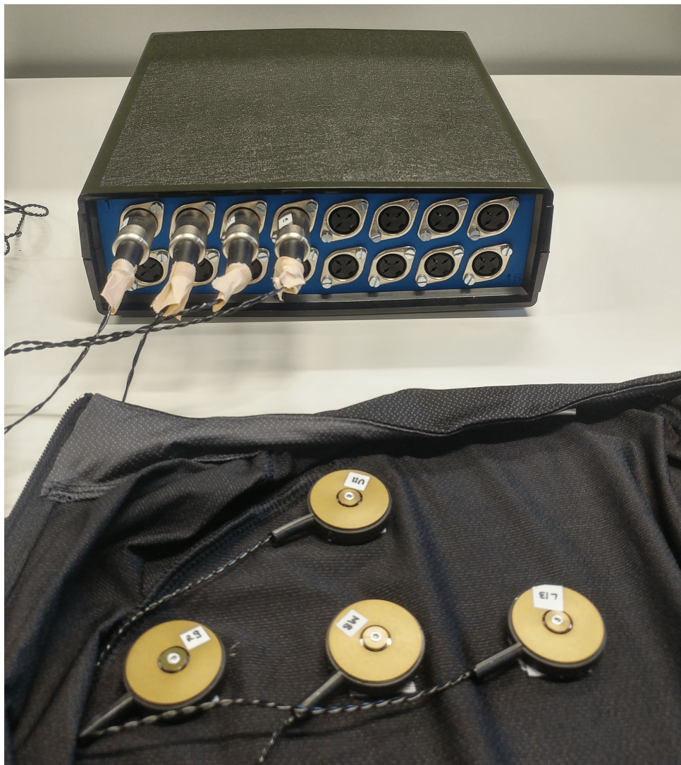
Figure 3.2: Four C-2 tactors attached to the inside of an elastic shirt and connected to an ARM Cortex M4 micro-controller.
