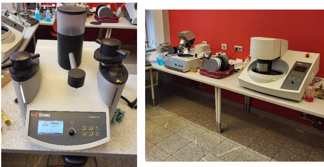
Figure 22. Struers Citopress 20 and Tegramin-30 machine for metallographic preparation
