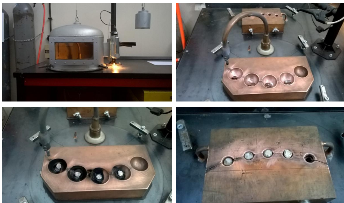
Figure 20. Processing of ingots in the electric arc furnace
