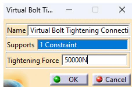
Slika 5.16 Virtual Bolt Tightening Connection Property
