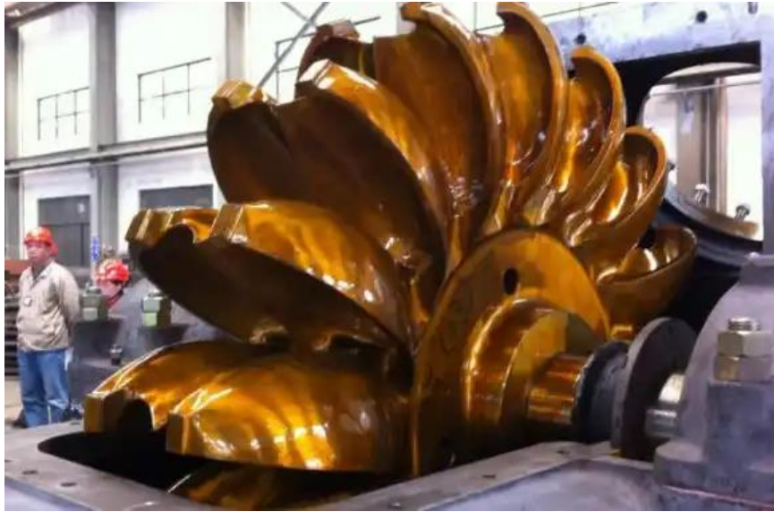
Slika 3.4 Lopatice Peltonove turbine [20]
