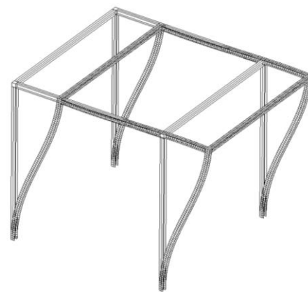
Figure 7. Sway buckling mode – shell model NASTRAN.
