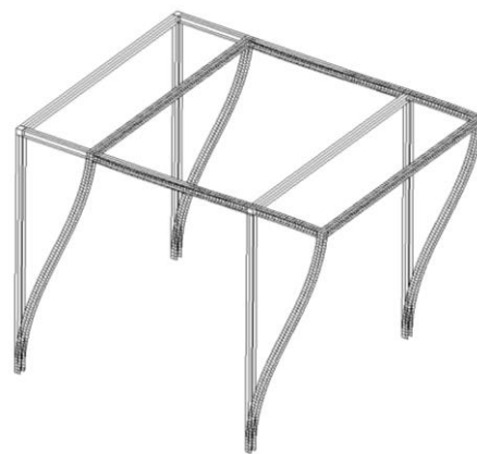
Figure 7. Sway buckling mode – shell model NASTRAN.
