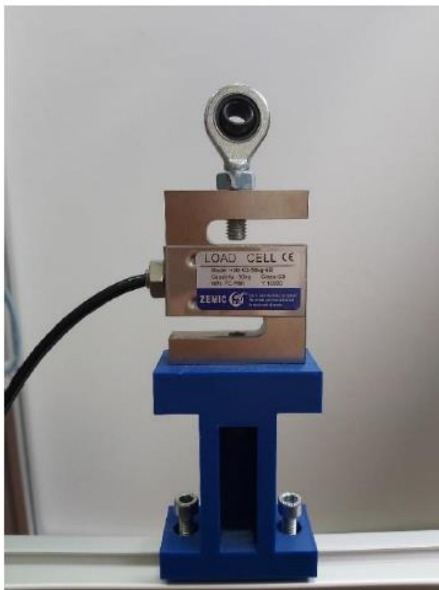
Slika 4.2.3. Senzor sile Zemic H3G-C3-50kg-6B [4]
